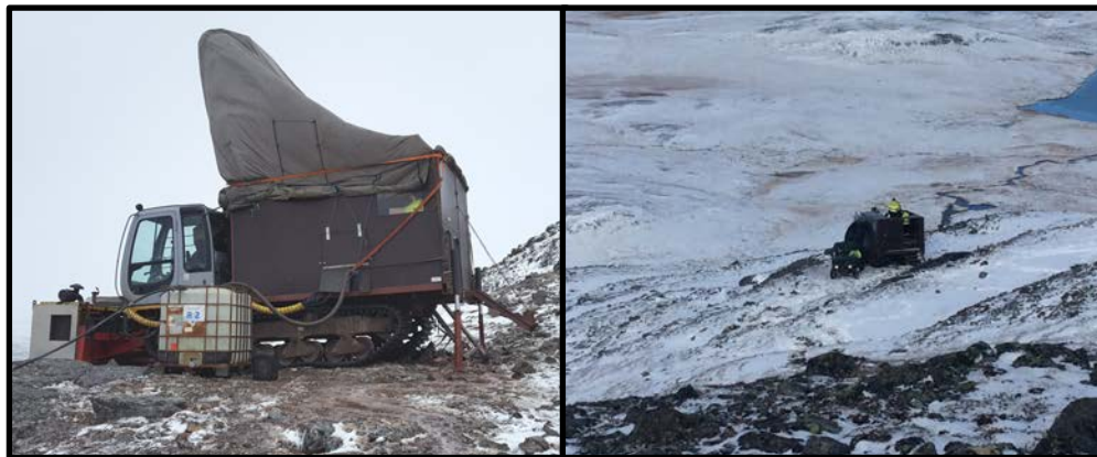
Figure 1. Winterized rig drilling mineralized outcrops at Burfjord.
